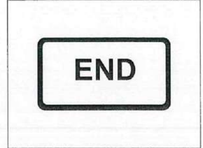
End of Construction, Sign RW41
