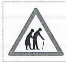
Old/Disabled People Crossing, Sign W71
